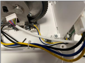
3. Slide the cable holder and tighten.
