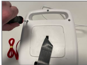
5. Remove screws from the bottom cover.
