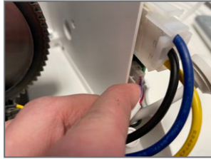
1.2. Remove the hand control connector.
