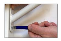
2. Drill the four holes in the cross beam with a 3,5 mm metal drill.
