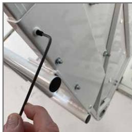
9. Screw on the Set Screw (3) with an Allen Key 3mm.
