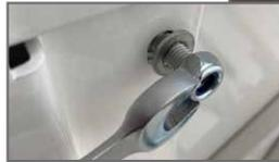
6. Place the two Screws M8 (4) in the inner holes of the backrest.
