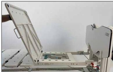
2. Unscrew the two screws with an allen key 3 mm.
