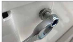
8. Place the Set Screw M6 (3) in the outer holes of the under side of the Care Assist Rail.
