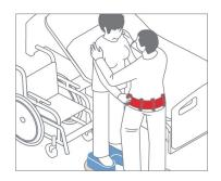
The Alpha Turning Disc can make transfers between bed and (wheel)chair easier for clients that are able to stand. The start and stop function of the Alpha Turning Disc allows movements to be precisely controlled.
