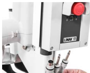
Checking wires connection
