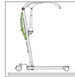
The Alzaro must only be used on a level surface clear of obstacles. Never use on stairs, escalators or an incline/decline such as up or down a hill.
