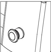
The emergency on/off push button will interrupt and stop the lifting process. For emergency lowering due to handset/button failure or power outage, the Alzaro is equipped with a manual emergency lowering system.
