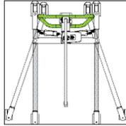
Bring the Alzaro up to the patient, spreading the base as required. Lock the rear casters. The patient should be facing the spreader bar.
