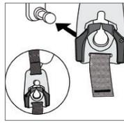
If using the self-balancing cradle, attach sling clips to Alzaro lift arm clips. Ensure all straps are straight and clips secure.
